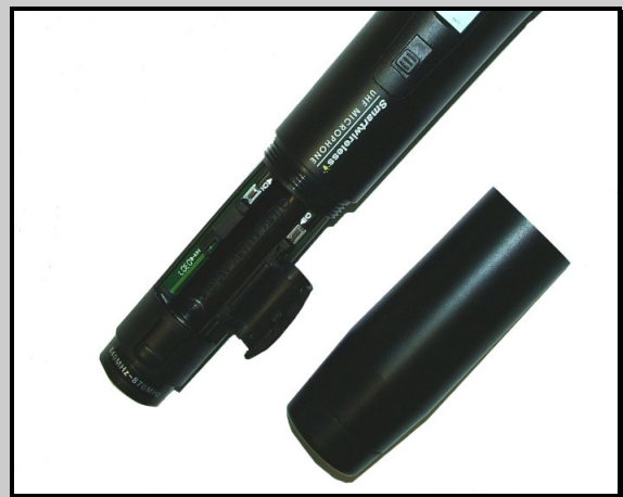
T1005/6 with the battery cover removed
